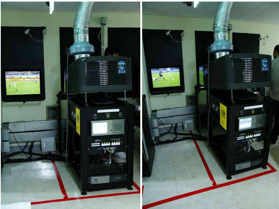
Equipment incorporated with GDC server at Lotte Hongdae Cinema for live 3D FIFA World Cup telecast.
